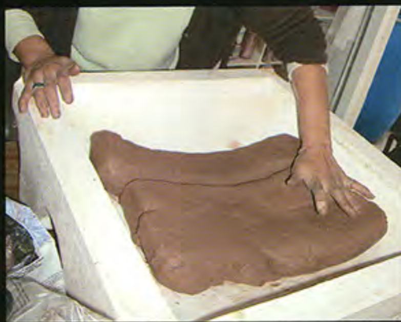
USING A FORMER: Clay is placed in plaster mould | Beating the clay to fill the mould | After levelling surface with metal kidney, depth of clay is measured with scribe.
