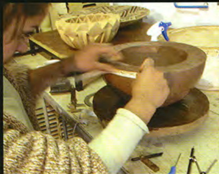
MARKING THE DESIGN: Water keeps surface of clay damp ■ Measuring circumference of bowl with tape measure ■ Using callipers and scribe to mark reference points.
