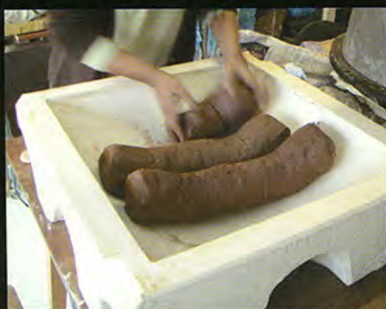
USING A FORMER: Clay is placed in plaster mould | Beating the clay to fill the mould | After levelling surface with metal kidney, depth of clay is measured with scribe.
